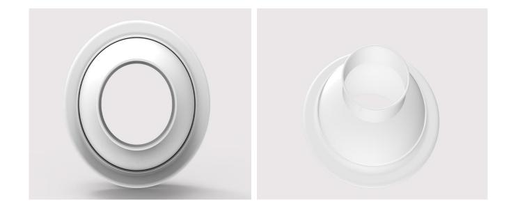
**AREAS OF USE AND FEATURES:** It is used as blowing diffusers in Hvac systems. It is suitable for vertical and horizontal use. The ideal shooting distance is between 3.5 m -15m. It is used for heating and cooling in sports halls, shopping malls, factory buildings and conference halls where high flow and long throw distances are required. Standard screw mounting. The way of mounting can be changed optionally.
